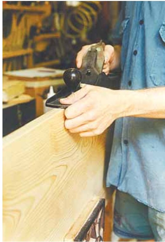
Use of hand plane to shoot the edge ready for jointing
