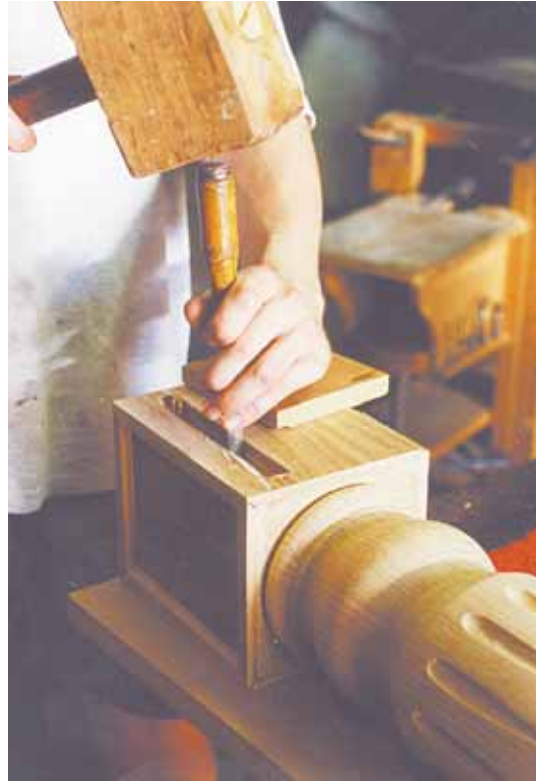
Chiselling out the mortise
