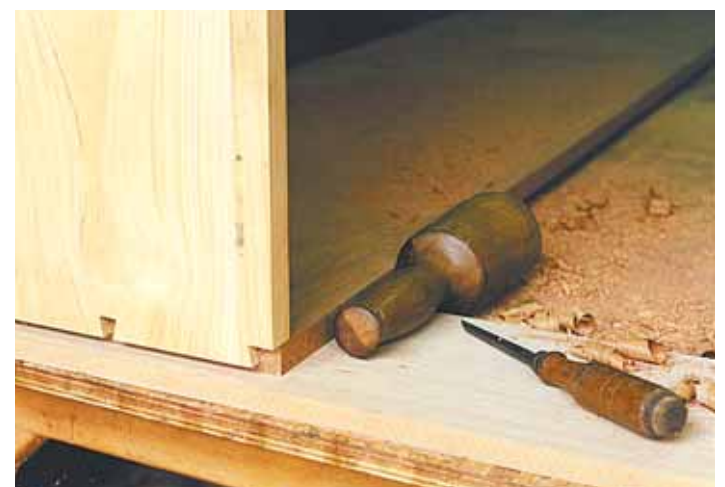
Dovetailing with mallet and chisel
