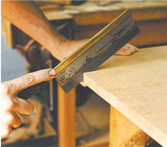
Dovetail joints made by hand using a dovetail saw
