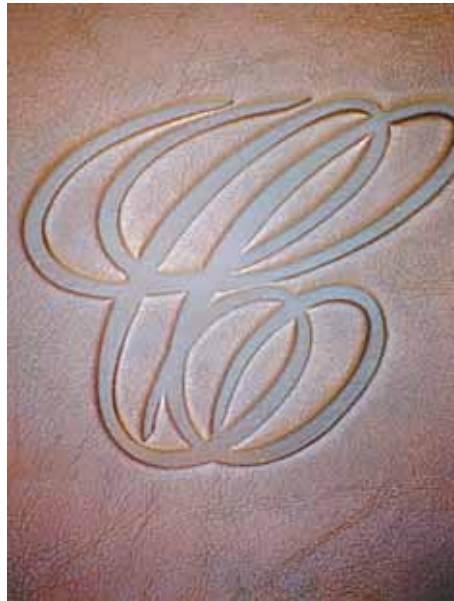
Corporate logos are embossed into leather for upholstery, panelling or desk inserts
