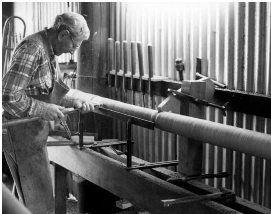
TOP: Jacobean table leg completed ABOVE: Arthur hand turning four identical oak Jacobean table legs which feature urns, tapering and square sections
